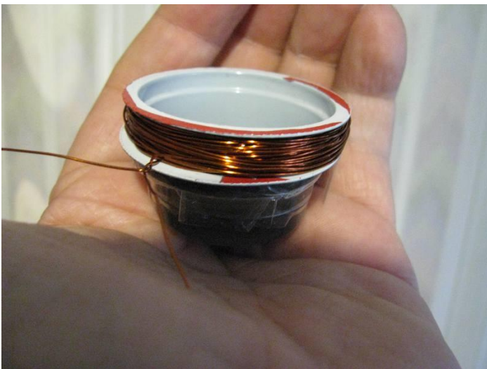
Fig 1. Coil wound on a "spool"
