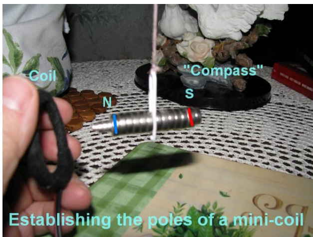
Figure 5. Establishing the poles of a mini- coil
