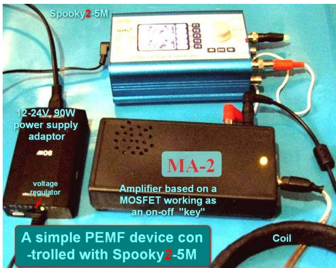
Ilustracja 4: A PEMF device I call MA-2 - connections of the key elements of the system
