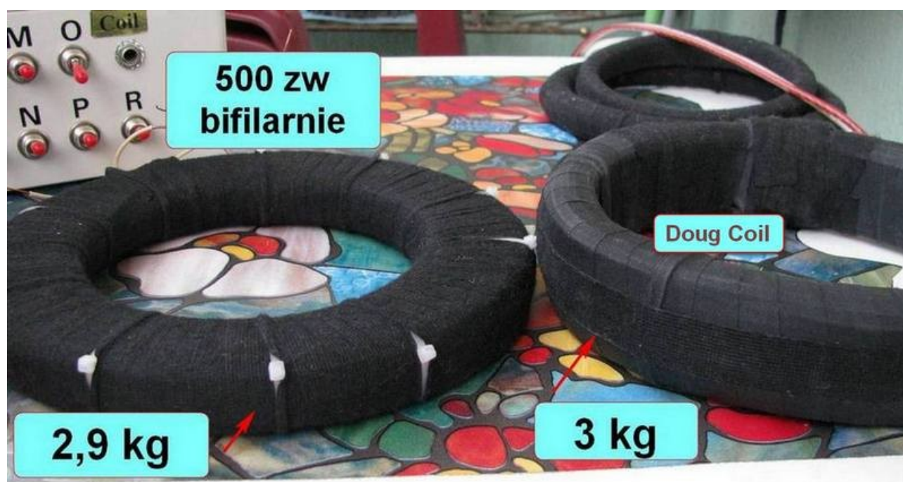
Ilustracja 2: Several coils, the Doug one presents just 1.4 Ohm resistance, the other ones about 7 Ohm.
