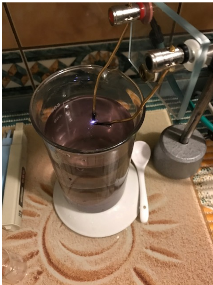
Illustration 1: HVAC method of making colloidal copper. The arc can be seen, just 2-4 mm under the surface of the water.
