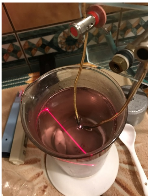
Illustration 4: Laser used - the red line proves the existence of metal copper particles in the batch.
