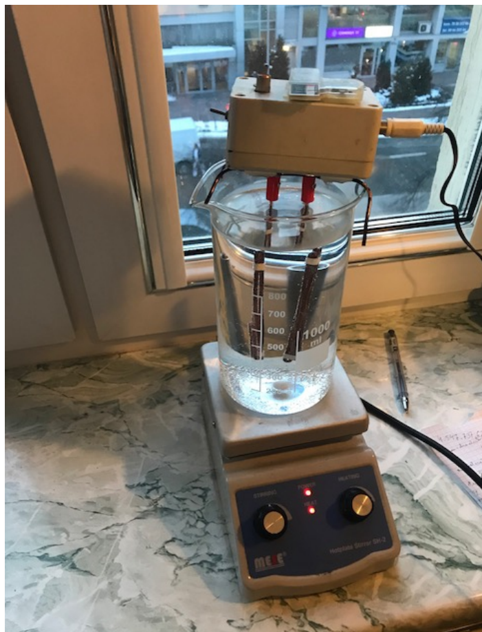
Illustration 3: LVDC method of making colloidal copper.
